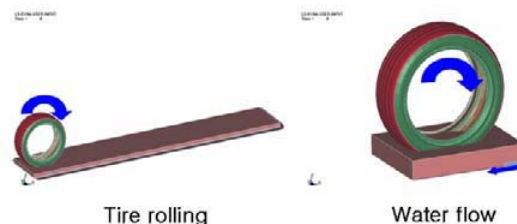
Fig. 8. Tire rolling and water flow models.
